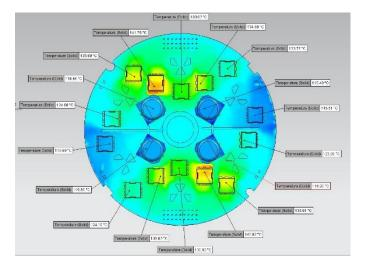
Contour plots of Temperature on the surface of a typical PCB and its components
