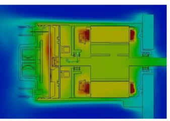
Contour plots of Temperature along motor axis for typical powerpack
