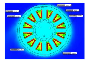
Contour plots of Temperature across motor axis for typical powerpack
